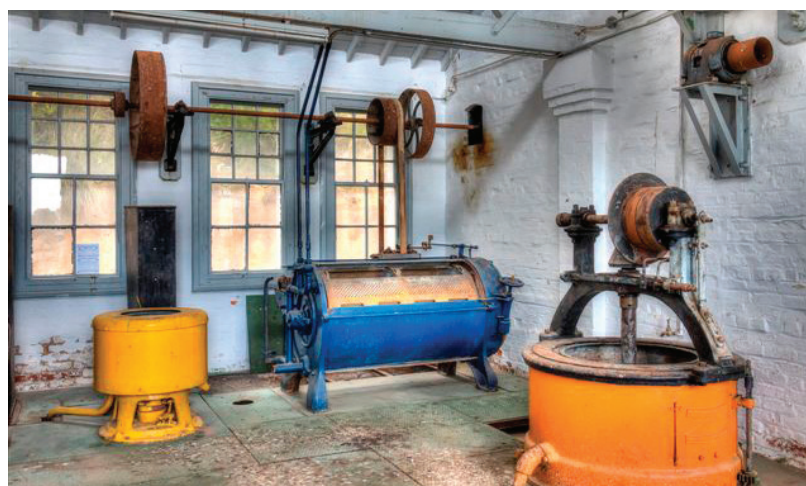
Fig. 3: Washing machine with horizontal drum and hydro-extractors. The original hydro-extractor is on the right. It was driven from the driveshaft that was later modified to be driven by a belt. This arrangement allowed the hydro-extractor to run at a higher, more efficient speed. The yellow machine on the left is a later hydro-extractor. The bright colours were applied when the area was used as a playroom for the children of a tenant. As part of the fun, the machines were filled with sand.
