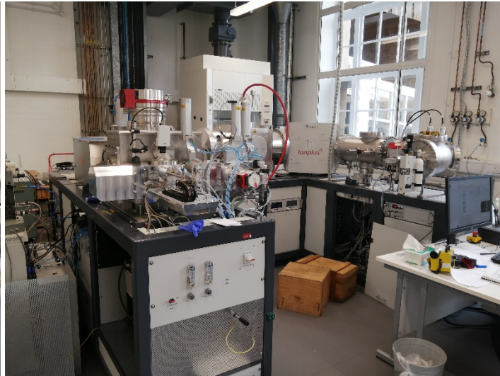
The line used to check the pressure in the graphitisation tube after combustion and the AMS
